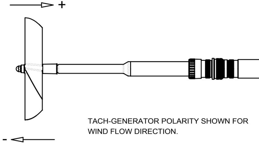
TACH-GENERATOR POLARITY SHOWN FOR WIND FLOW DIRECTION.
